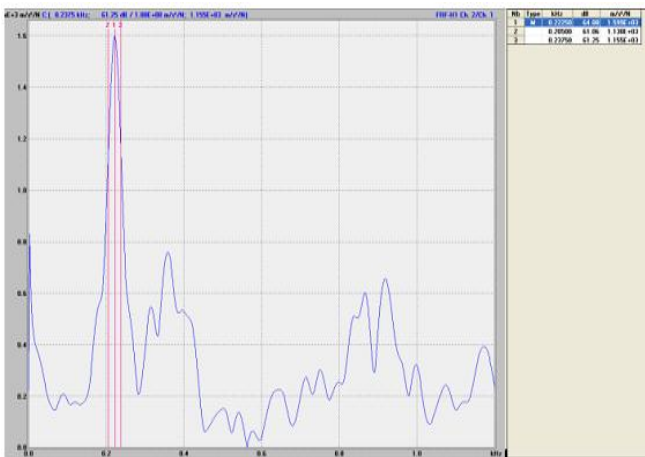
Figure 8: Natural frequencies for damping ratio of hemp/epoxy composite with 0% cenosphere
