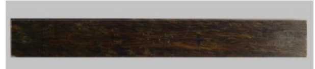
Figure 3: Hemp/Epoxy polymer composite specimen for vibration test
