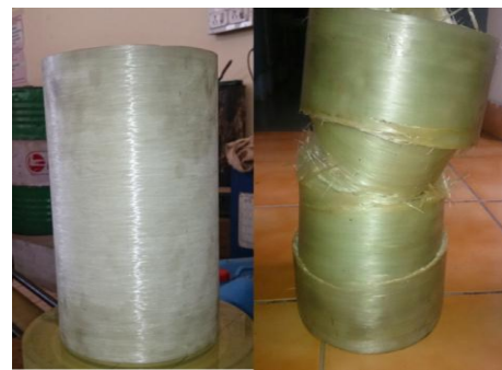
Figure 3.2 Glass/Vinyl ester cylinder before buckling And after buckling respectively
