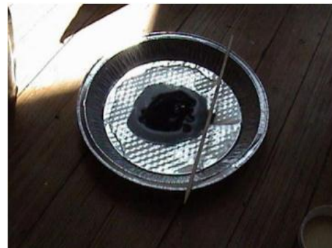
Fig 4.12: Addition of ink into the oil
