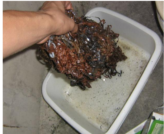
Fig:4.7: Placing tapes in the bowl containing acetone
