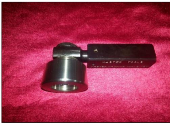
Fig.3 Roller burnishing tool
