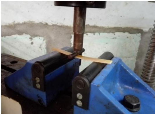
Fig.5 : Specimen loaded for bending test
