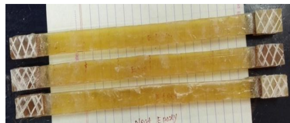
Fig.4 : Tensile Specimen with tabbings at the end
