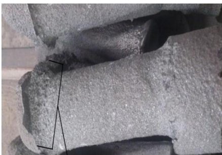
Fig 5 showing sand inclusion in return metal
