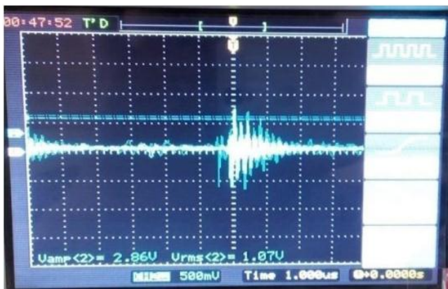
Fig.14 Output waveform during step down conversion ( V_o=3V )
