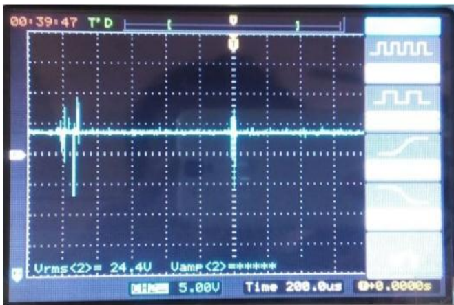
Fig.13. Output waveform during step up conversion ( V_o=25V )
