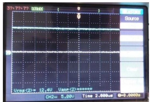
Fig.12. Input voltage waveform (Vin=12V)
