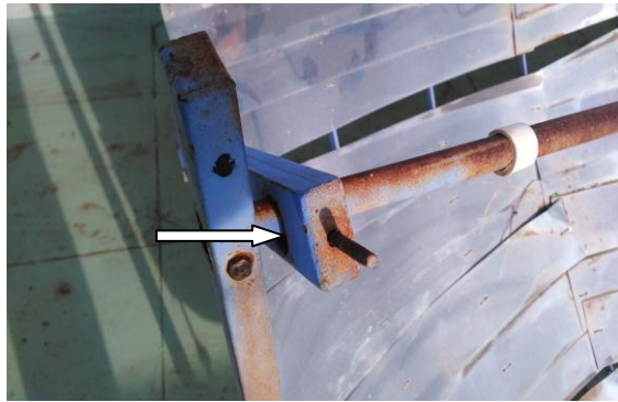
Fig.3 Concentrator not focused
