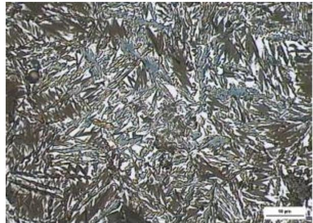
**Fig. 5. Microstructure of specimen after isothermal heat treatment – 380°C/ 60', ADI – matrix created by upper bainite and retained austenite [14].**
