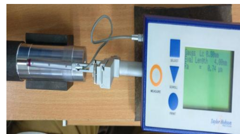
Fig.8 Surface roughness measurement using surface tester
