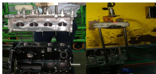
Fig.6 (a) Assembly of head on block with guide tool
