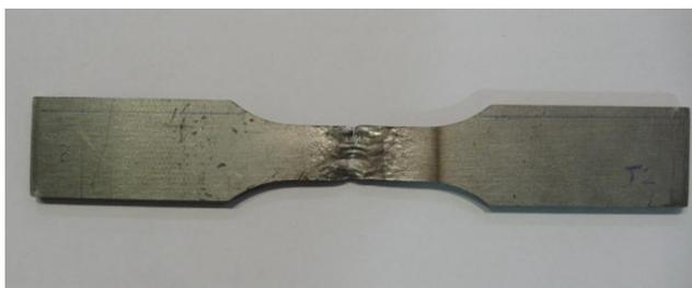
**Fig. 4 Tensile test specimen after testing**
