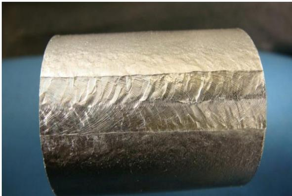
Fig. 6 Guide bend specimen after testing
