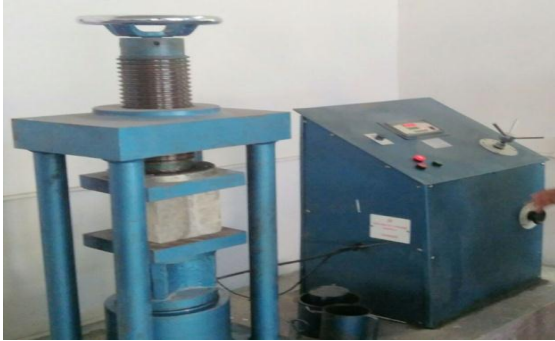
Figure 3: Compressive Testing Machine
