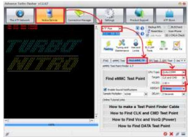
Figure 2: ATF software setup for eMMC Test Point Identification
