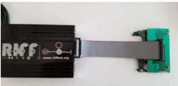
Figure 8: Samsung Galaxy S4 I9505 connected to Riff Box via jig
