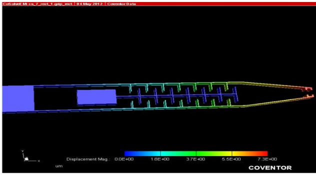
Figure 1: FEM simulation of the pull-in analysis in Coventor Ware
