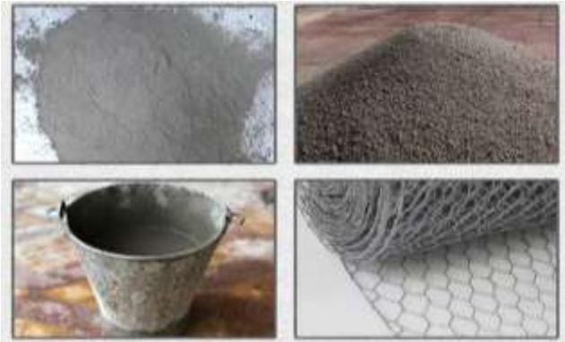
Fig 2: Ferrocement construction materials
