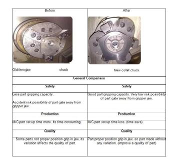
Table 3: Provide collet chuck for gear turning department
