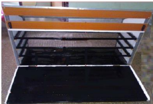
Figure 3: Dryer with the Trays Loaded in Position
