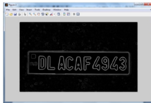
Figure 6. Extraction of Number Plate Location (II)
