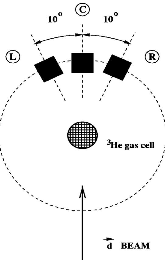
The beam current was integrated from the gas cell and a tantalum foil in front of the  $0^\circ$  detector. Calculations with were performed to obtain the beam energies corresponding to the mean reaction energies at the center of the gas cell. This procedure was also used for the self-supported targets described later in Sec. II B.
