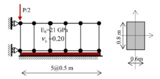
the impact of soil properties on interaction response The mechanical properties of the beam and the ground are stated in Fig. 16. In horizontal direction, a fne mesh is chosen but vertically a
