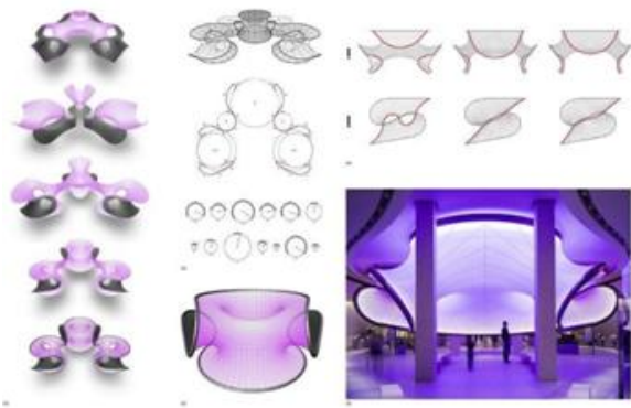
Figure 8: The mathematics gallery has eight fabric constructions. 01 A rapid CAGD methodology allows for several design revisions. 02 The edge-pipes might be bent physically thanks to bespoke CAGD equipment. 03 Layout of seams (in collaborations with Base Structures and Mark White). 04 CAGD and Engineered Geometries are compared. 05 The structure has been completed. (Photo credit: Zaha Hadid Architects)
