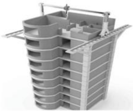
Figure 1 : Gantry system Printer with multi-storey construction
