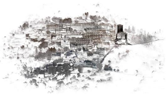
View of the town of Campi di Norcia. The elaborate has been obtained from the union of the scans made with the Leica P40 laser scanner
