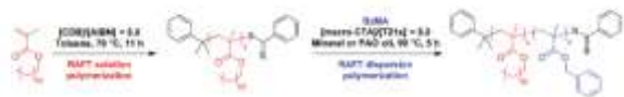
Fig. 1 Synthesis of a poly(lauryl methacrylate) macro-CTA via RAFT solution polymerization in toluene at 70 °C, followed by RAFT dispersion polymerization of benzyl methacrylate (BzMA) in mineral oil or a poly(α-olefin) (PAO) at 90 °C
