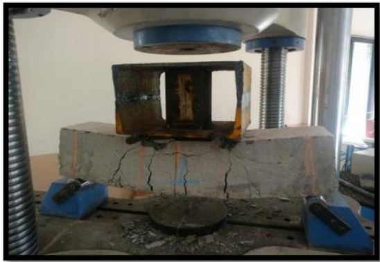
Fig 4.2: Beam under Four Point Loading
