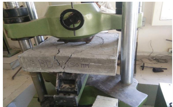
Fig.4 Crack patterns in Bubble deck slab.
