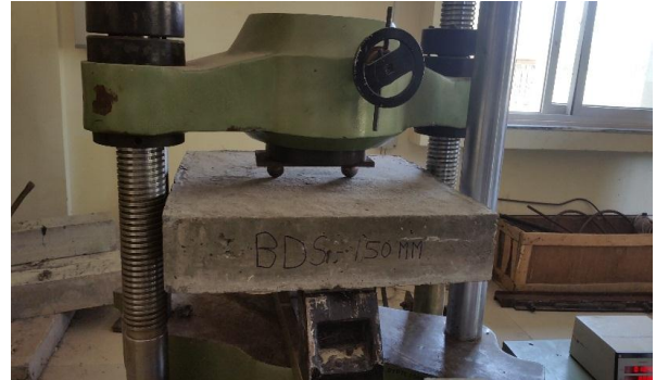
Fig. 3 Two-point loading by using metal balls.
