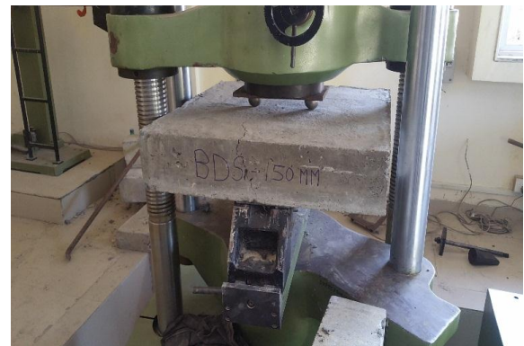
Fig. 3 Two-point loading by using metal balls.
