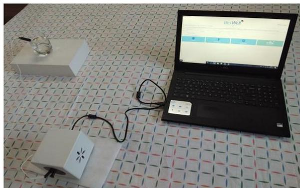
FIG 1- SYSTEM SETUP (LEFT TO RIGHT) WATER SENSOR, BIO-WELL CAMERA AND WINDOWS COMPUTER LOADED WITH BIO-WELL SOFTWARE
